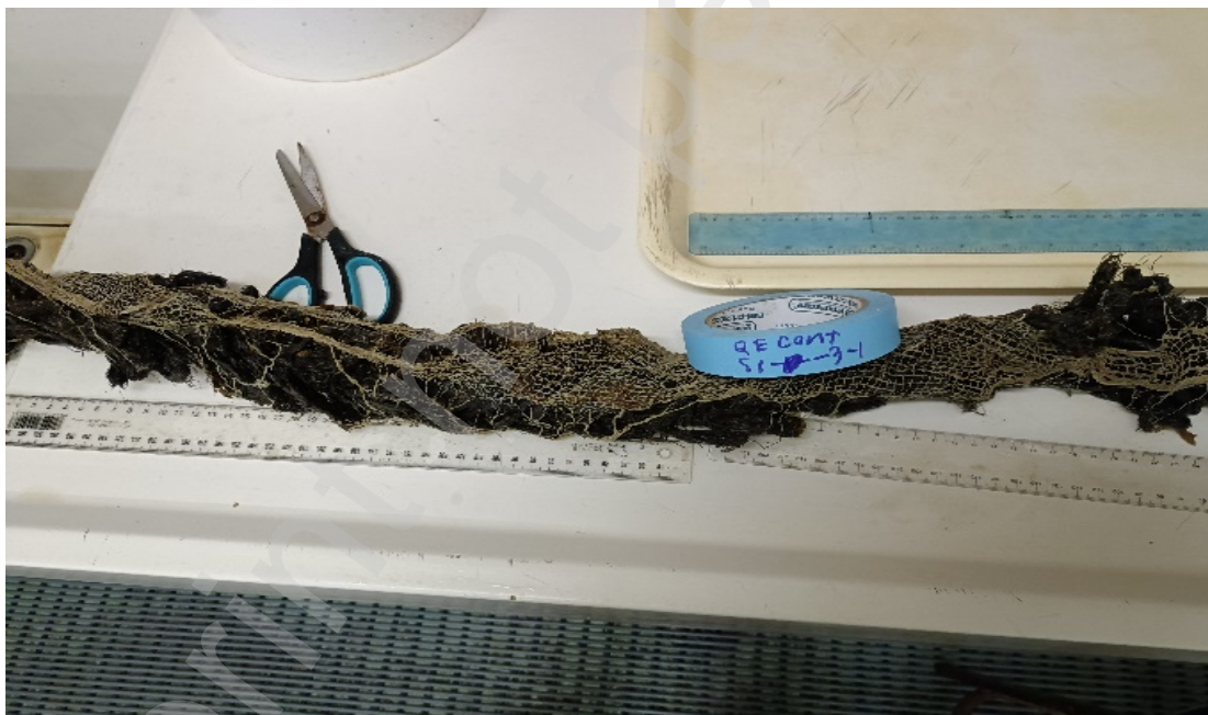
516 517 Fig. 6. A section of the Control Standard Polycotton stocking after 12 days (Sample 1), showing the 518 extent of the tearing in the stocking from fish predation activity on the encased mussels.
